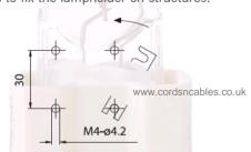
Fixing of the lampholder by M4 or M3 screws, to be inserted in the fixing holes, of the spring bracket, with center distance 30 mm.
